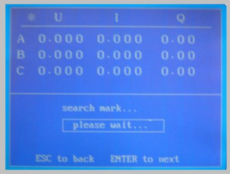
If 'Search mark' function is enabled(in system ParaSet), embedded software will process 'Search mark' function firstly, if 'Search mark' function is disabled, this screen won't display.
