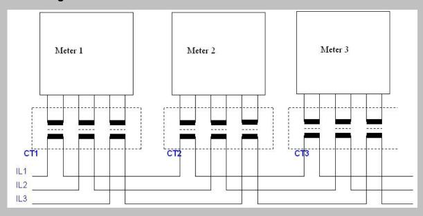
From the digram, it shows the current for every tested meter is isolated by the ICT, the current supply to the meter from the output of every ICT.
